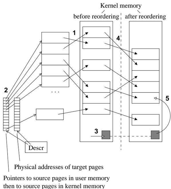
Figure 15: Booting: memory reordering in the kernel.
