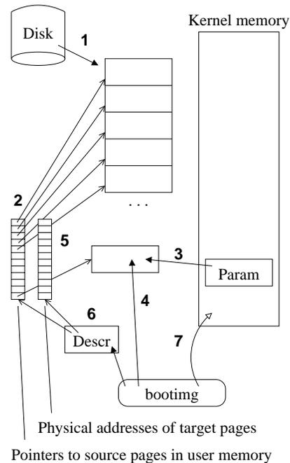
Figure 14: Booting: set up from user space.
