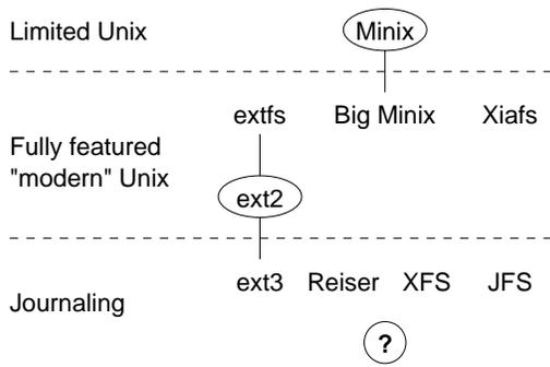
Figure 6: Evolution of the “standard” Linux file system.
